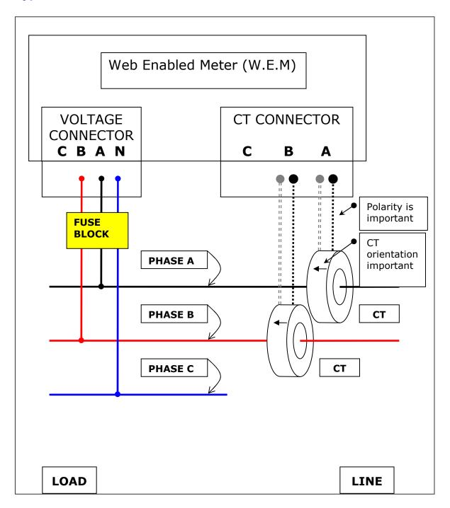
Application: Measurement of Output from Solar Inverter.
